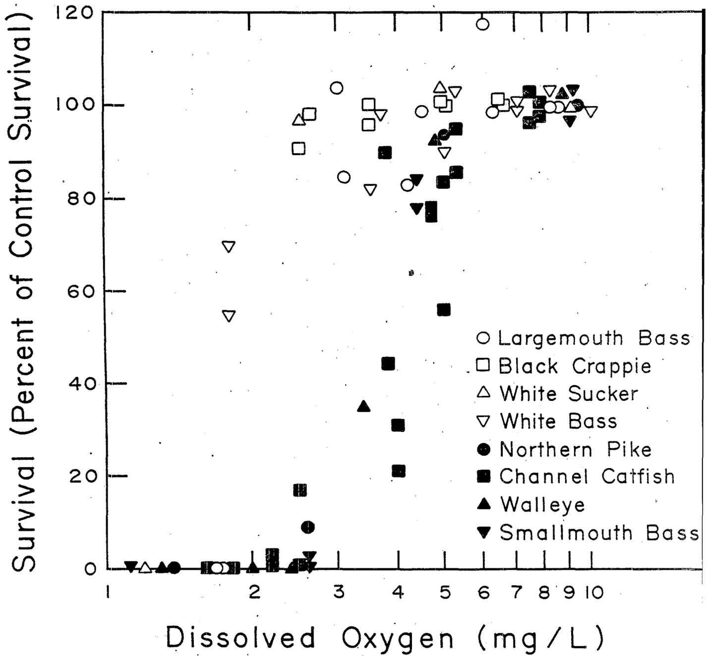
Figure 1. Effect of continuous exposure to various mean dissolved oxygen concentrations on survival of embryonic and larval stages of eight species of nonsalmonid fish. Minima recorded in these tests averaged about 0.3 mg/l below the mean concentrations.
