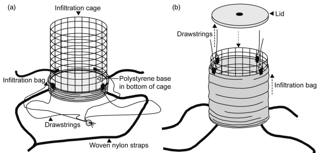
Figure 2. The infiltration basket, showing (a) the infiltration bag folded around the base of the infiltration cage and (b) the infiltration bag partially pulled up around the sides of the infiltration cage and the Perspex lid
