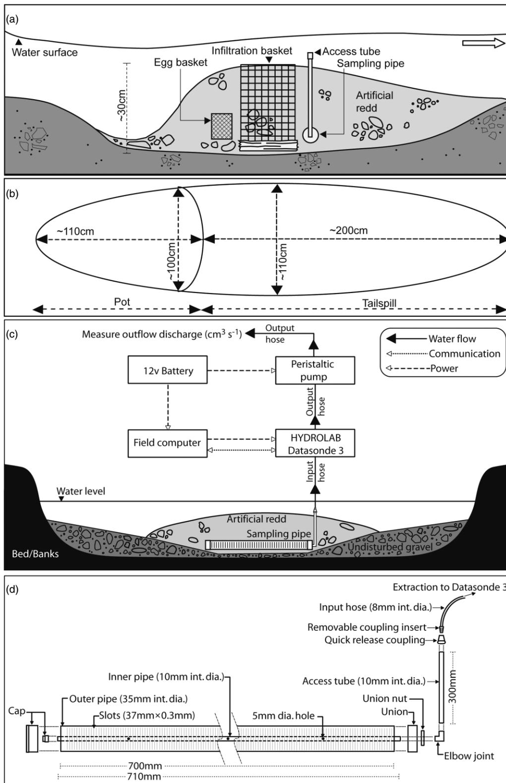
Figure 3. Details of the redd sampling strategy showing (a) a schematic representation of a longitudinal section of an artificial redd depicting the installation of an egg basket, an infiltration basket and an intragravel water sampling pipe, (b) a plan view of an artificial redd showing its approximate dimensions, (c) the approach used for intragravel water sampling and (d) the intragravel water sampling pipe and its components
