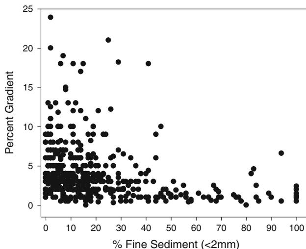
**Fig. 1** Percent fine sediment (<2 mm) and stream gradients
