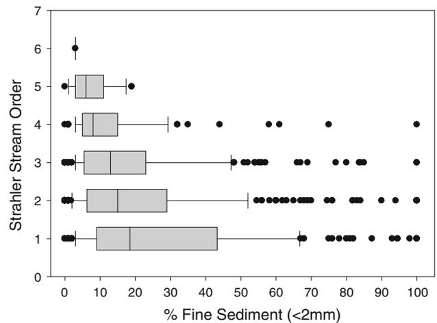
**Fig. 2** Percent fine sediment (<2 mm) at different Strahler stream orders ( $n =$  first—172, second—292, third—207, fourth—88, fifth—27, sixth—1) Box plot median is vertical line, box ends the 25th and 75th percentiles, error bars the 10th and 90th percentiles, and filled circles represent full range of data
