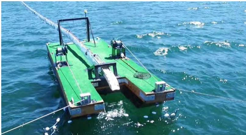
Fig 8. Fish exit barge configured for single Migrator™ tube.
