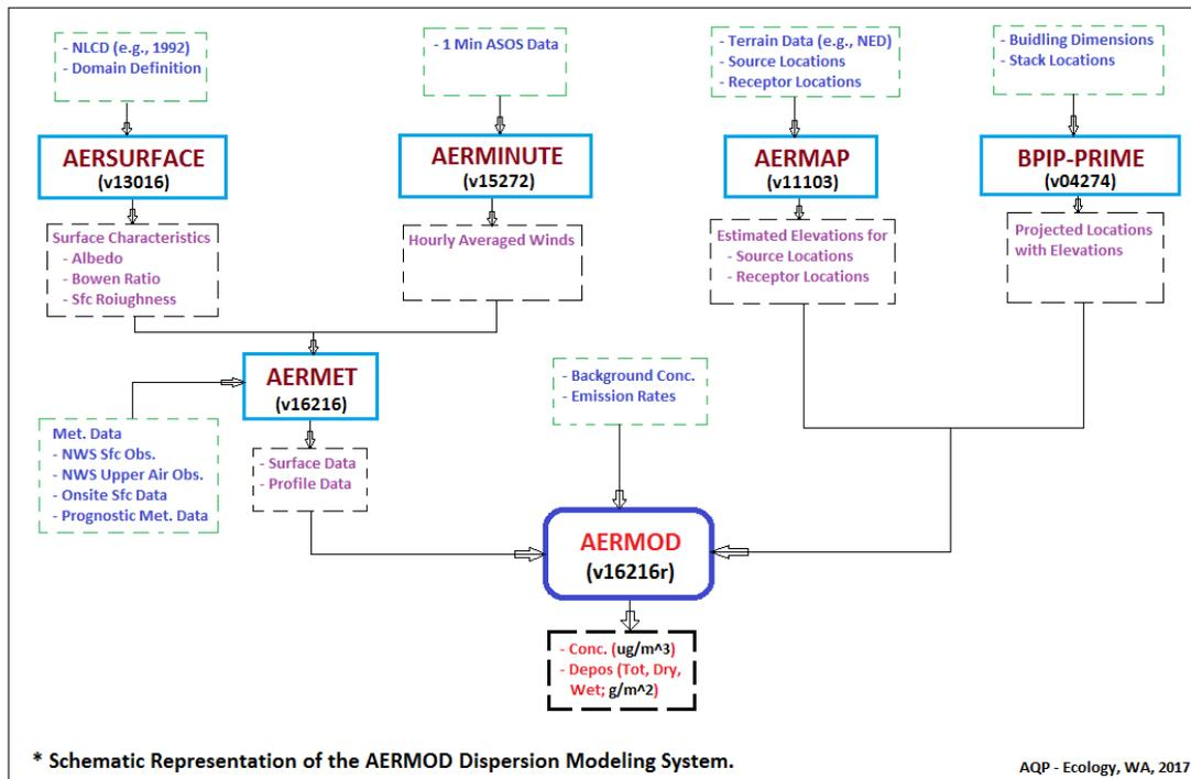
Fig. 2. The AERMOD dispersion modeling system (with program versions) is depicted schematically, with the required input data for each suit program and their expected outputs.
