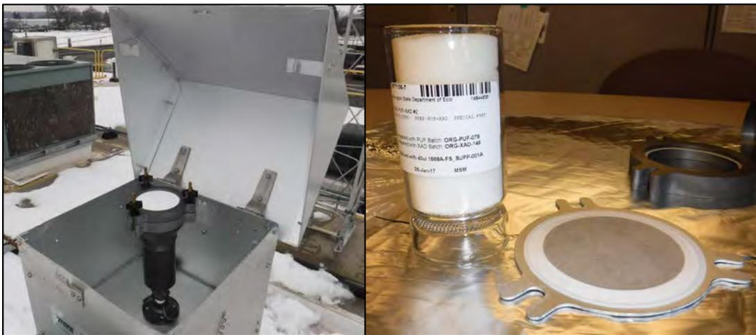
Figure 5. PUF sampler head (left) and PUF glass cartridge and filter sample (right).
