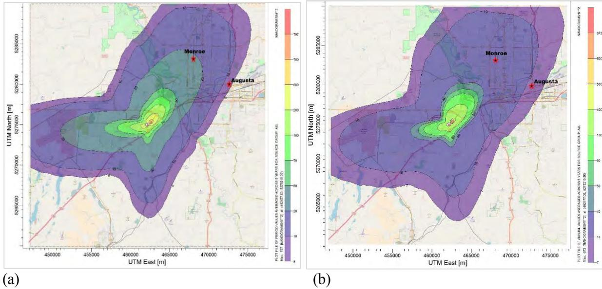
Figure 16. Modeled average annual total (bulk) deposition distribution from the Spokane WTE stack. (a) For May 11, 2016 to May 11, 2017 field measurement case study. (b) Regulatory 5-year modeling study period of January 2011 to December 2015. Coordinates are in UTM (m) and deposition is in nanograms per square meter ( $ng/m^2$ ).
