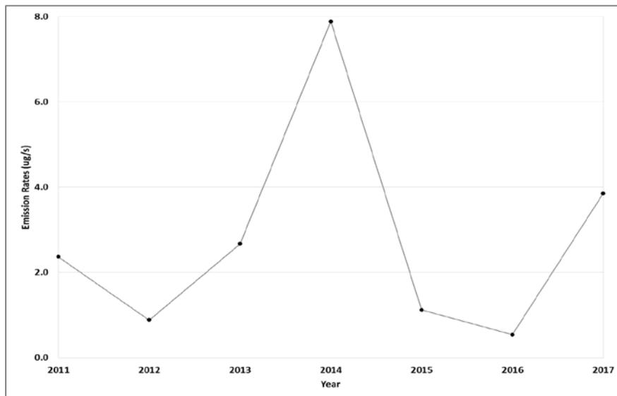
**Fig. 4.** Spokane WTE Facility single-unit emission rates estimated from measurement runs for 2011 through 2017 using eq. 1.
