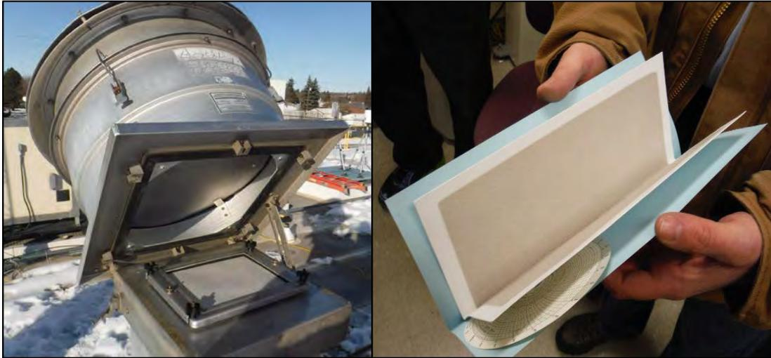
Figure 4. PM10 sampler head (left) and PM10 filter sample (right).
