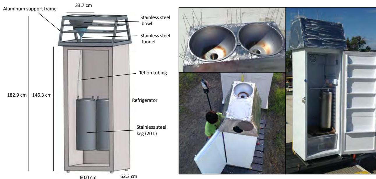
Figure 3. Schematic and Pictures of Bulk Deposition Sampler.
