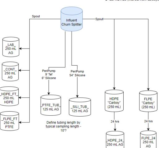
EACH SAMPLE = ~ 13<u>L into churn splitter</u> Fresh Tubing?!?! 6 125-mL AGs direct 2 1.5-gal carboys (fresh?) 2 125-mL AGs (indirect from carboys)
