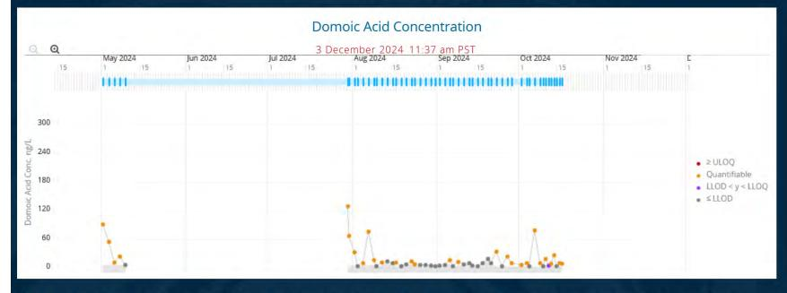
Concentration of particulate domoic acid in seawater. Domoic acid is a toxin produced by some species of phytoplankton in the genus *Pseudonitzschia*. If domoic acid concentrations are detected above the Lower Limit Of Quantification (LLOQ, see description below), this means that one or
