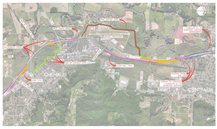
Figure 2: Alternative 1 - I-5 Levees and Walls, Raise Airport Levee, New SW Chehalis Levee
