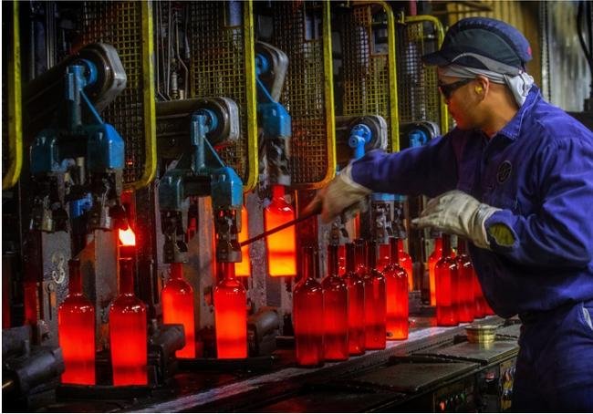
Marvin Diego, an individual section machine operator, works at Ardagh Group's Seattle facility. Ardagh Group operates a plant where 130 tons of cullet — recycled glass fragments — are melted each... (Ellen M. Banner / The Seattle Times) [More](#) ▾
