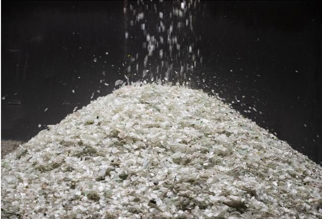
Crushed glass called cullet drops off a conveyor belt onto the apex of a 15-foot-high pile at Strategic Materials in Seattle. The Sodo facility sorts, cleans and tumbles fragmented glass from... (Ellen M. Banner / The Seattle Times) [More](#) ✓
