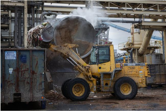
A heavy-equipment operator picks up garbage ejected from the pulping vat at NORPAC in Longview. The garbage was mixed in with the paper and cardboard that are being recycled. Twenty truckloads of... (Ellen M. Banner / The Seattle Times) [More](#) ✓
