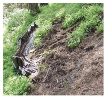
Elk trampling and animal digging caused much of the erosion measured in the study plots.
