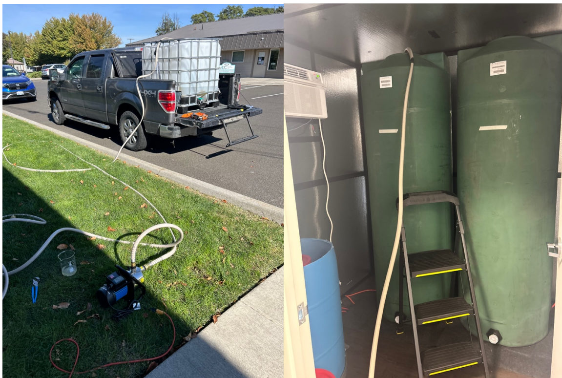
Figure 6. Transfer of screened wastewater from the IBC transport container (left) into the facility cold storage tanks used to preserve wastewater at 4°C prior to dosing into the RAV systems (right).
