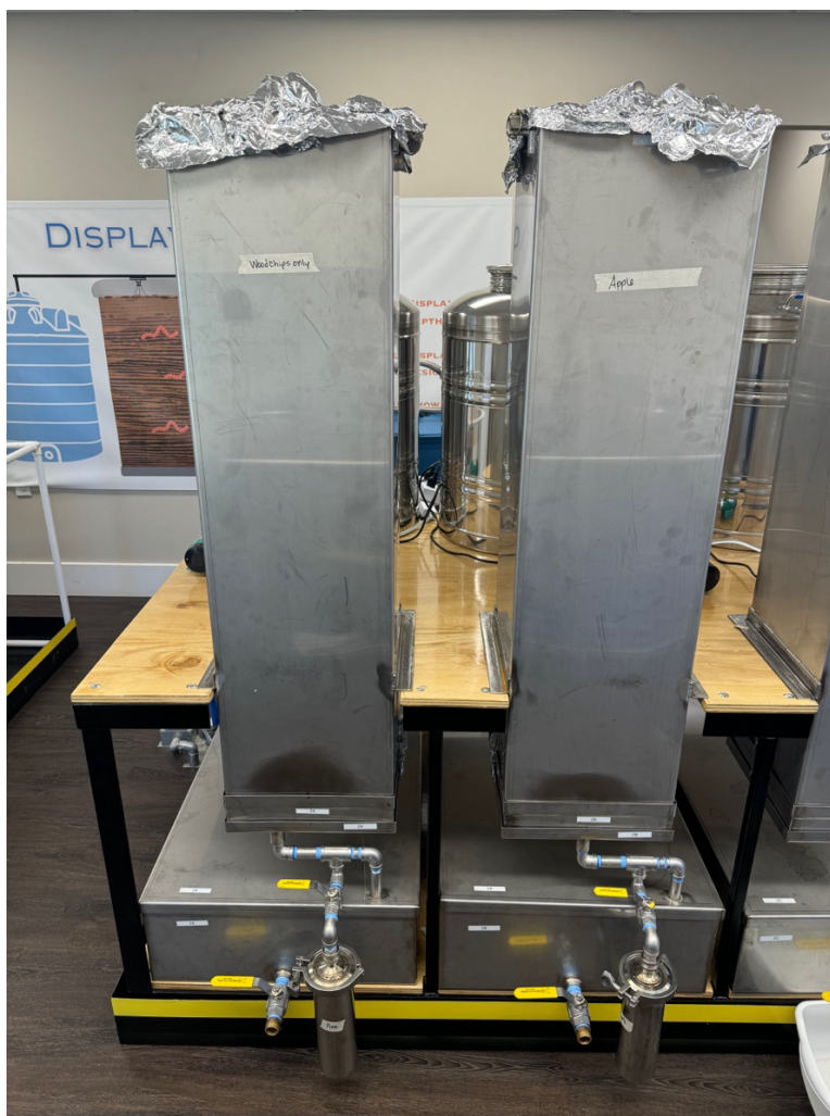
Figure 7. Rapid Assay Vermifiltration (RAV) systems used for bench-scale testing containing traditional organic media (left) and apple wood fines (right).
