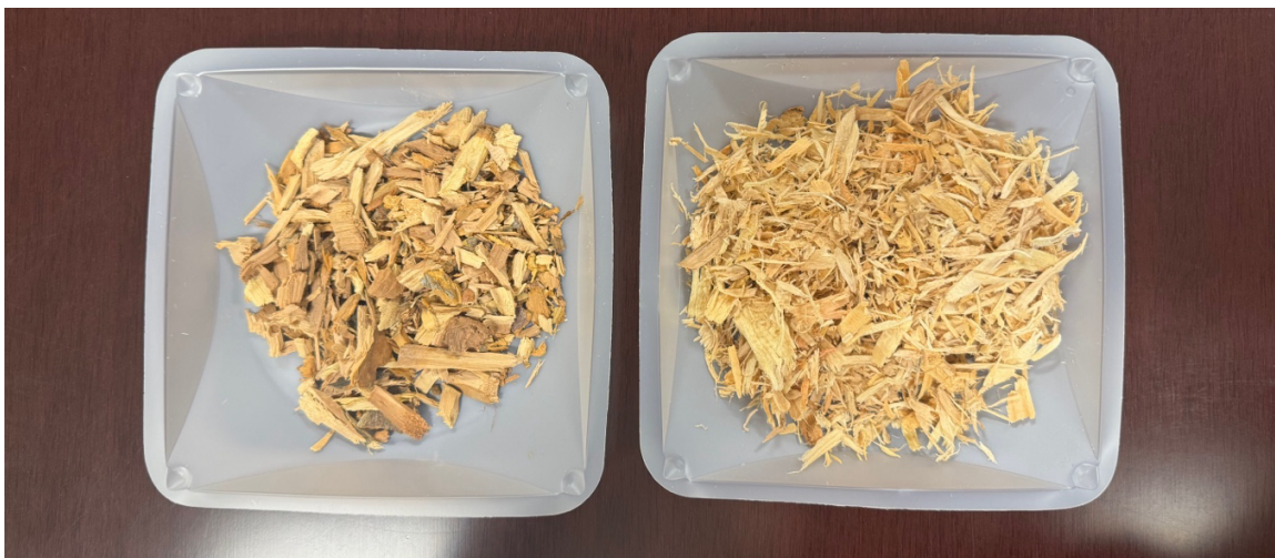
Figure 5. Apple wood chip fines (left) and traditional, conifer-based organic media (right) used as substrate materials in bench-scale vermifiltration testing.
