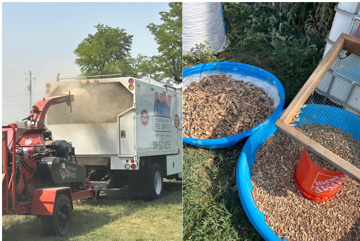
Figure 3. Industrial chipper processing orchard tear-out wood (left) and manual screen used to separate fines (<½ inch) from oversized material for use as vermifiltration media (right).
