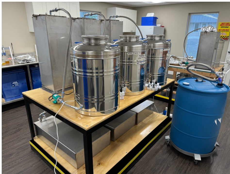
Figure 8. Transfer setup used to load refrigerated wastewater from cold storage into RAV source tanks.
