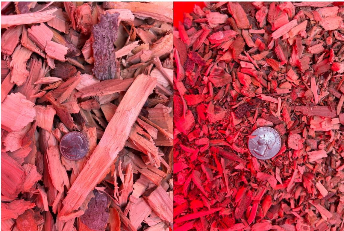
Figure 4. Oversized wood chips (>½ inch) discarded from the screening process (left) and retained fines (<½ inch) used as substrate media in vermifiltration testing for this study (right).
