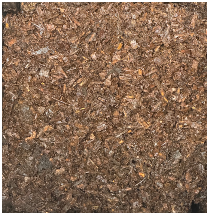
Figure 15. Upper third of the apple wood media bed at the conclusion of testing, showing high earthworm activity and visible saturation compared to traditional media.
