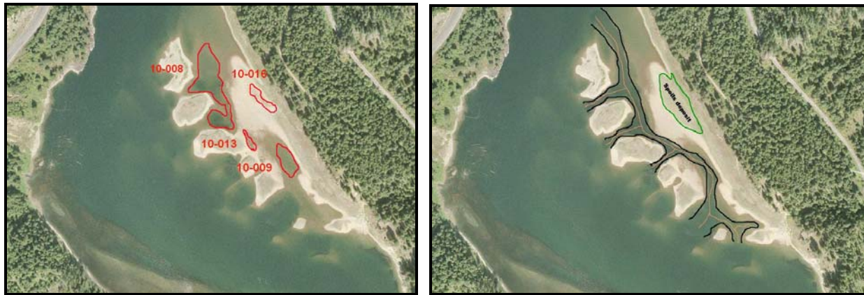
Figure 5.1-2. Location of trapping pools (left) and conceptual plan (right) for modification at Cobble Sisters.
