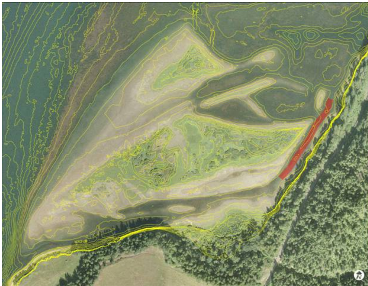
Figure 3.2-3. Proposed location of macrophyte bottom barrier Fish Stranding and Trapping Region 9 (PRM 28.8). Area shown in red indicates the proposed location of the bottom barrier.
