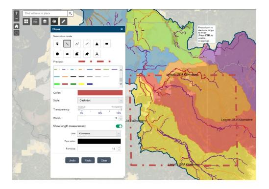
Select an icon under draw mode to begin drawing. A straight line, polyline, or curved line can be useful for redefining areas or showing a certain extent, as shown in this example. Adjust the line symbol. In this example, the "Show length measurement" option is toggled on (in kilometers). If you would like to share a map with a drawing, take a screen shot. **Once you navigate away from this map, your drawings will disappear.**
