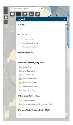
Only layers that are checked "on" in the layers list and are visible in the current map extent will be displayed in the legend. To change what is shown in the legend, uncheck items and zoom in/out until all desired layers are visible in the map.
