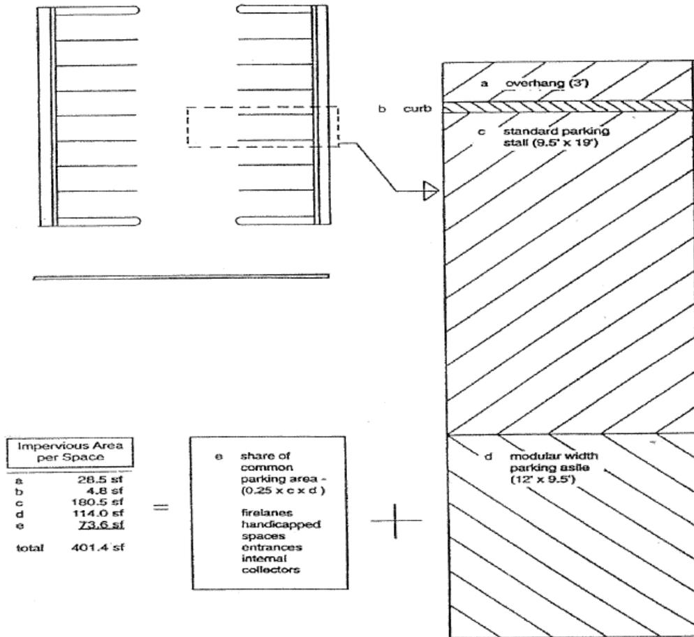
A parking stall is supported by a larger parking space that includes the (a) overhang, (b) curb, (c) stall, (d) parking aisle needed to get into the stall, and (e) the stall's share of common parking area, such as entrances, internal collectors, fire lanes and handicapped parking spaces. When these extra features are added in, the approximately 180 ft<sup>2</sup> needed for each parking stall increases to over 400 square feet.
