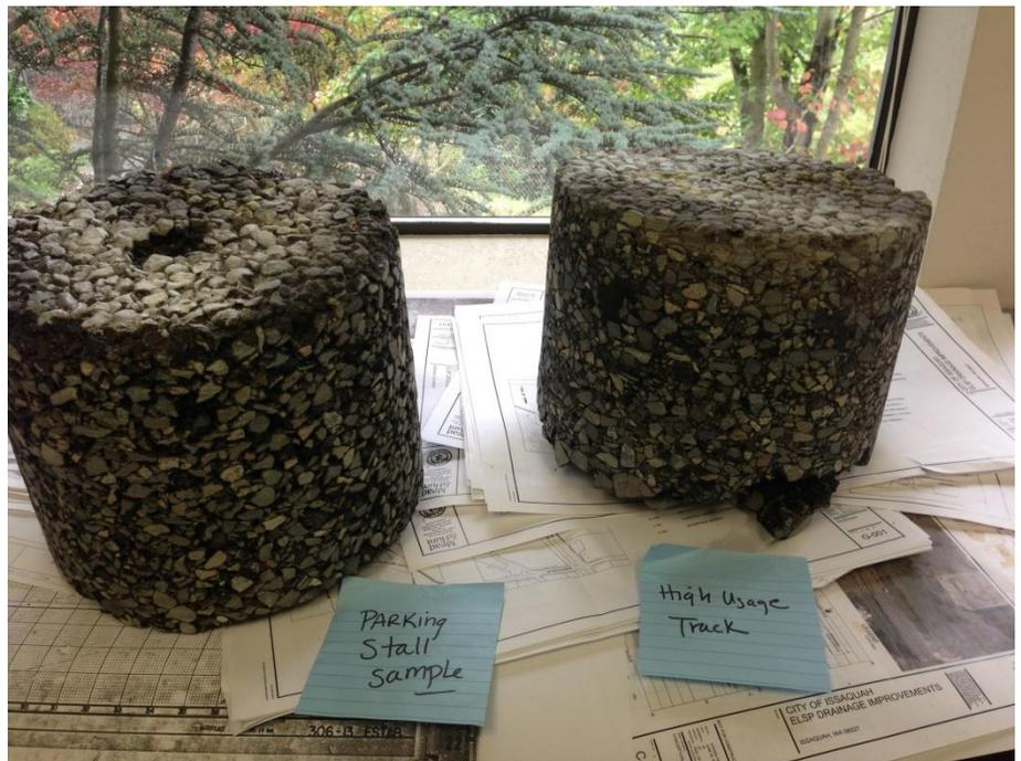
**Figure 4. Cores from permeable pavement installations in Kirkland. Core on left is from a parking stall. Core on right is from roadway with heavy usage. More particulate matter is imbedded in the voids in the heavy usage core.**
