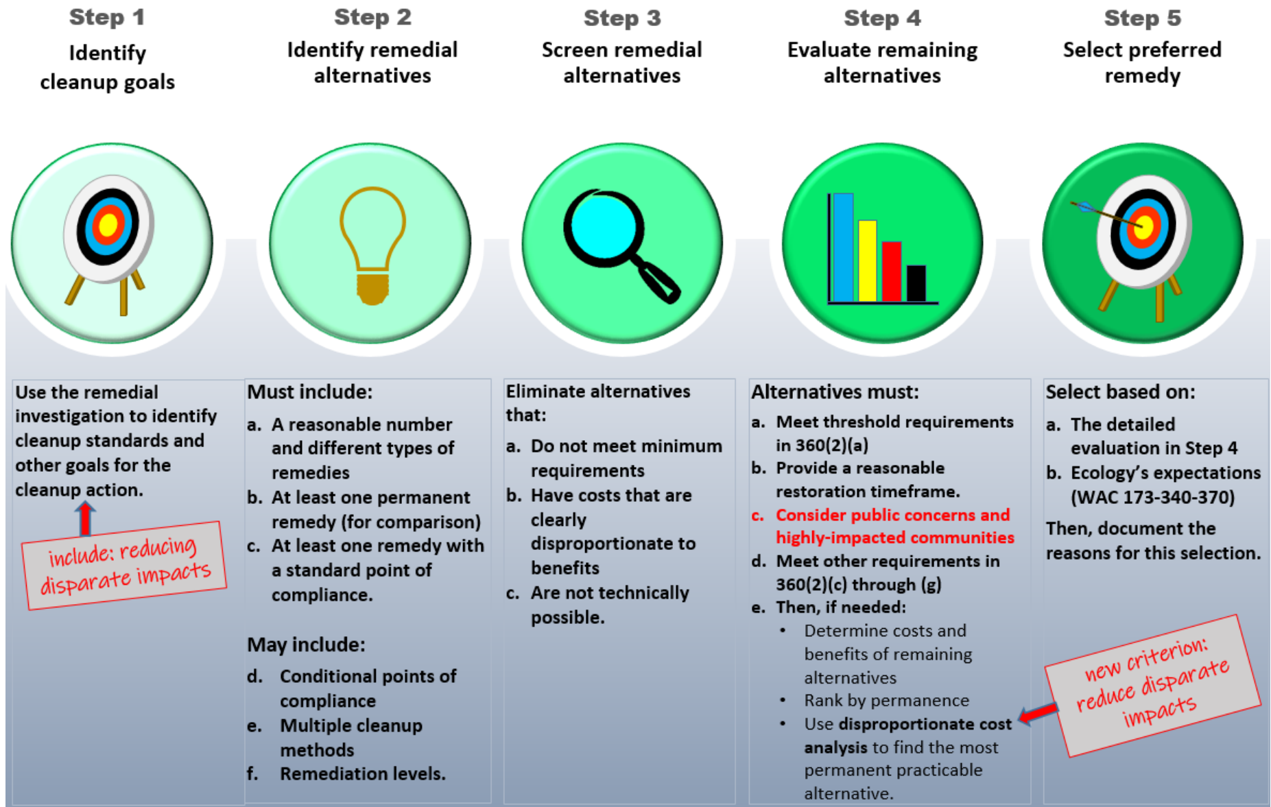
Figure 1: Remedy selection process under WAC 173-340-350 and 173-340-360
