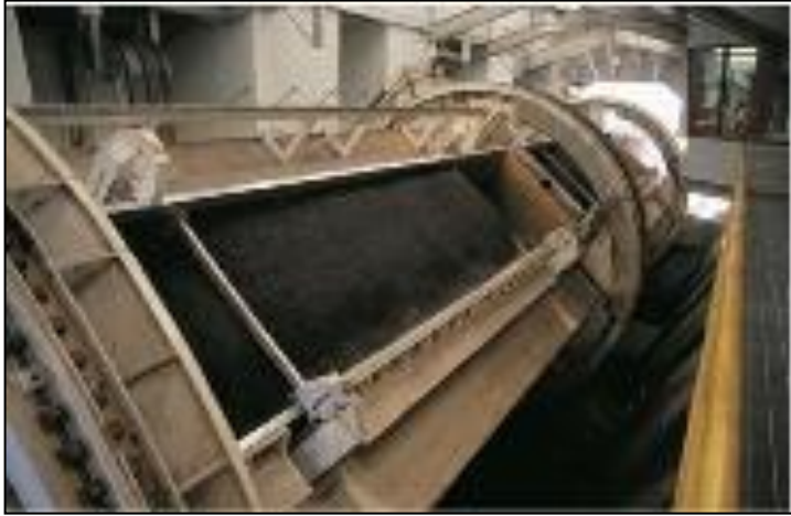
Tandem Rotary Dumper (Coal within a Shed, Woodchips Outside)
