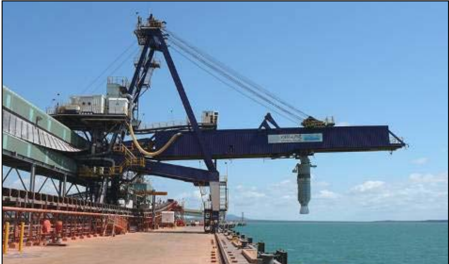
Shiploader with Enclosed Gallery & Enclosed Boom
