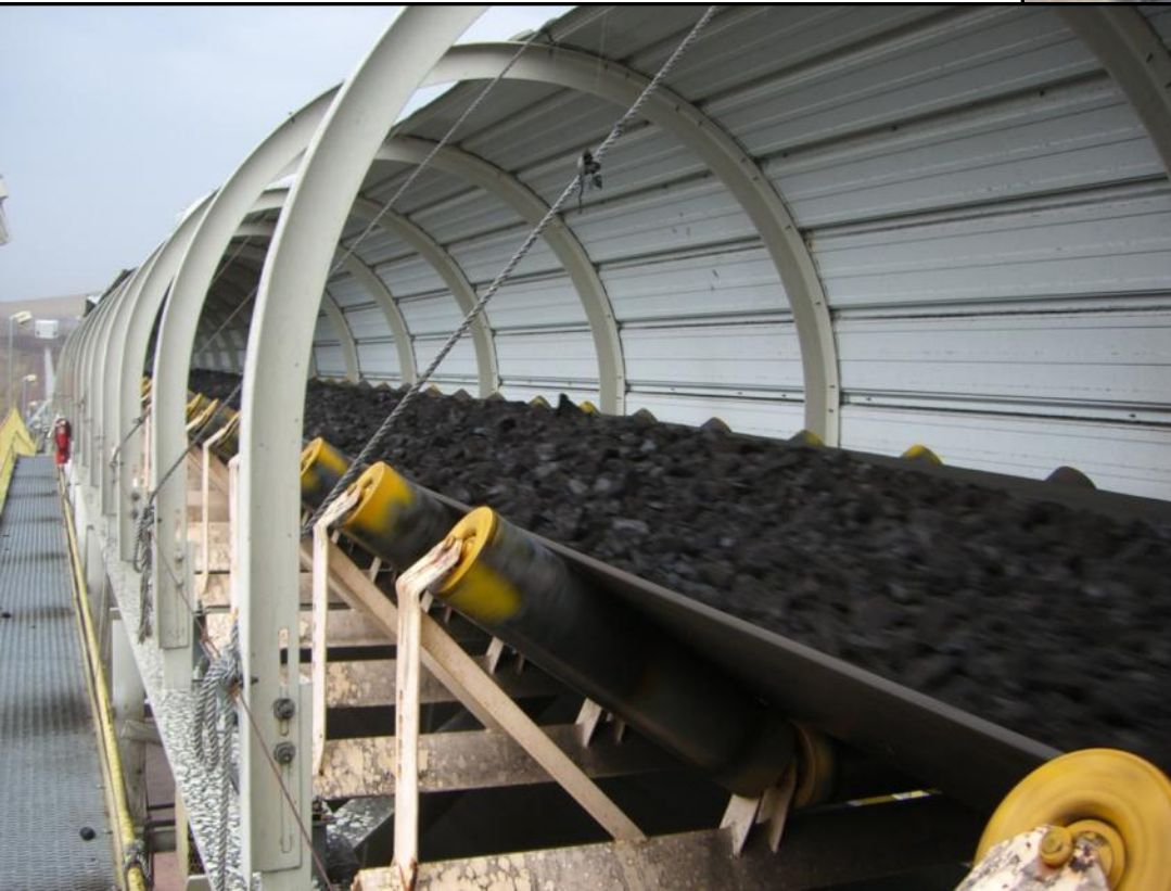
Half Covered Conveyor (shown to illustrate the conveyor inside)
