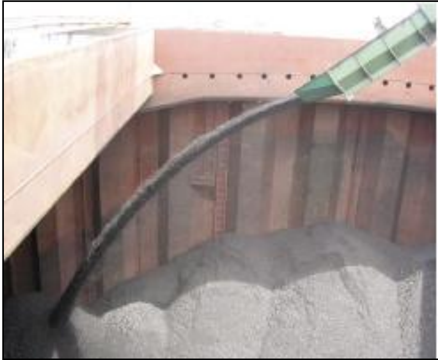
Example of Banana Spout Loading Coal Vessel
