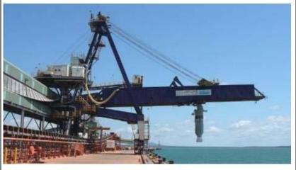
Over Water Conveyance – Open Conveyors and Shiploader
