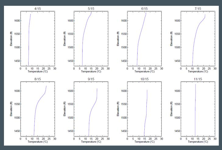
• Model simulated the dynamics of thermal stratification successfully
